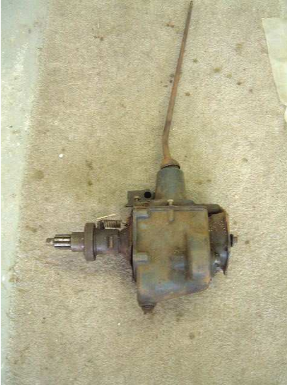
Photo of Model A transmission with throw-out bearing, bearing carrier, and pull back spring in place. Note the flange on back (right) end of the transmission that bolted to the rigid Model A driveshaft housing. (It gets cut down to facilitate installation.)
