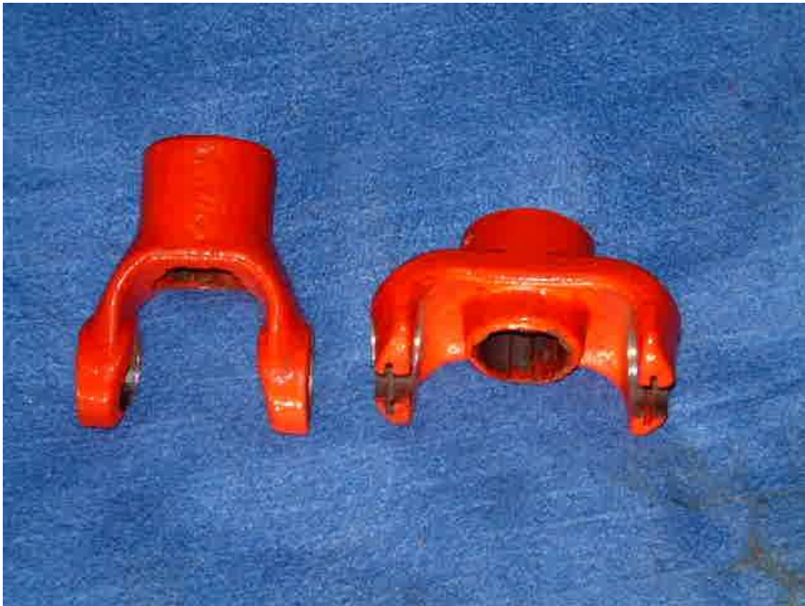
Photo of the HG U-joint yoke (left) and the Model A U-joint yoke. Note the length difference.
