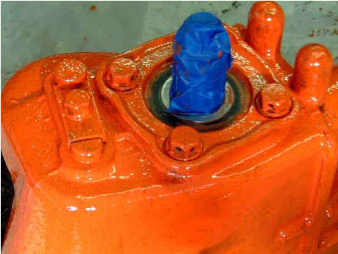
Photo of transmission rear output shaft bearing retainer with outer flange cut off. The open shaft splines (hidden by the masking tape) must be sealed to the bearing to prevent oil loss.
