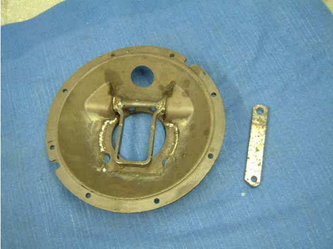
Photo of the clutch release yoke welded to the 1/2 inch diameter actuating rod inside the clutch cover. Note that the lever to the right of the assembly is too long. The pivot holes in it should be (4 5/8 inches) the same distance apart as the top pivot rod is from the holes in the side of the yoke near the bottom, to ensure the clutch peddle pressure and lever travel are correct. After this picture was taken, a new lever was made. (No the material is not gold. The color results from fluorescent lighting and incorrect camera settings.)
