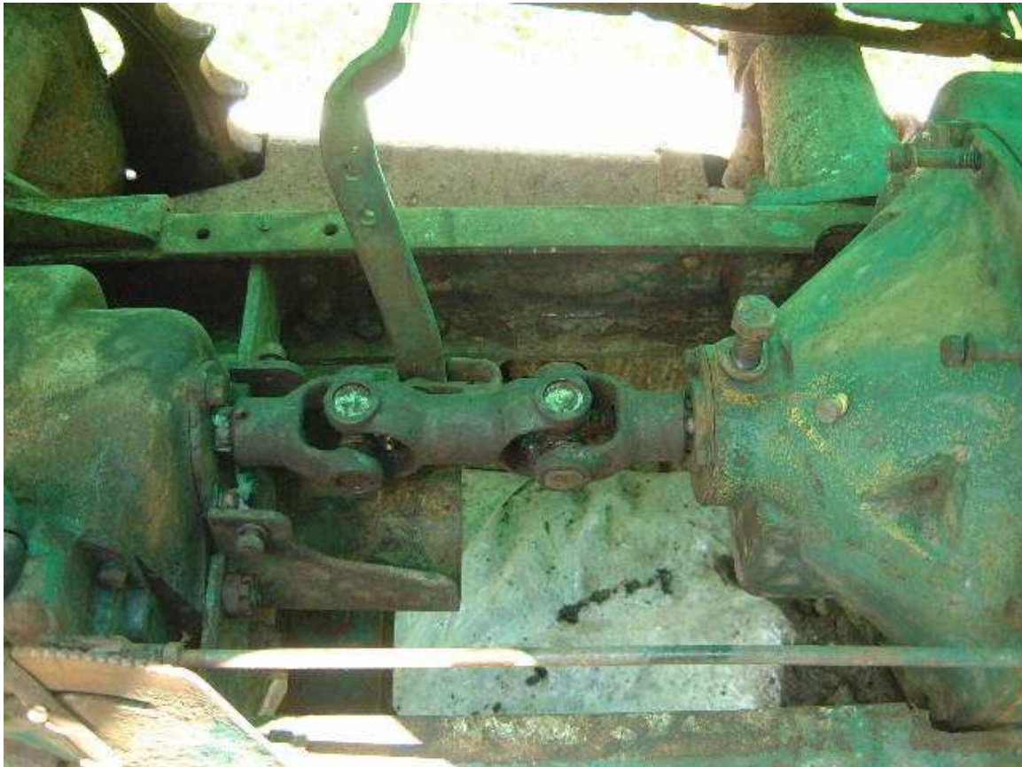
Photo of stock HG drive shaft with U-joints and yokes at each end.
