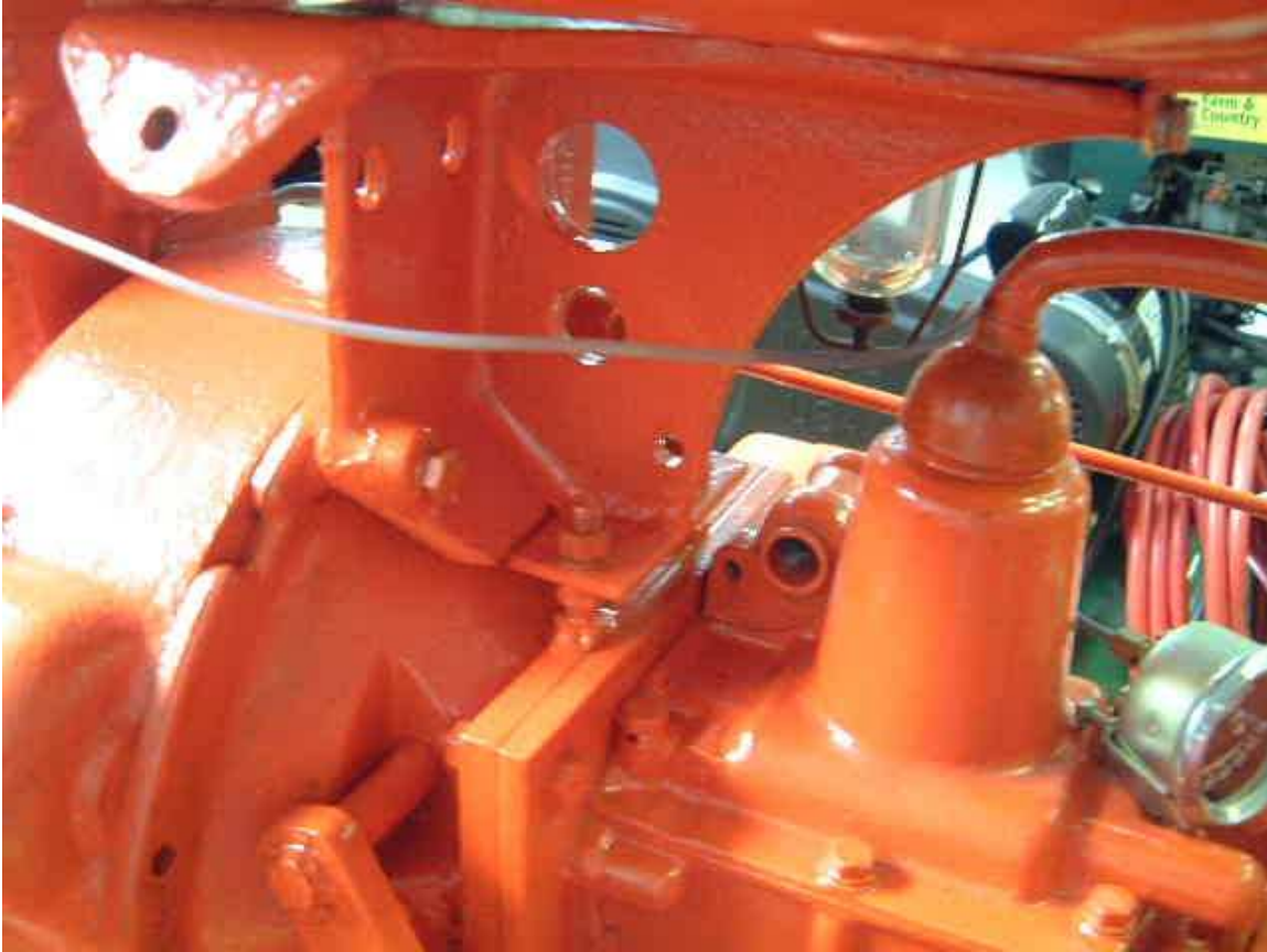
Photo of modified gas tank support bracket installed. Note location where original was cut.
